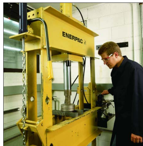
◀ An Enerpac H-Frame press makes quick work of removing the shaft from this assembly.
